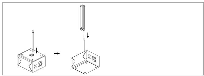
STEP 2: Please insert the pole-mount on a subwoofer base socket and insert the pole-mount in the column "B" pole-mount socket
