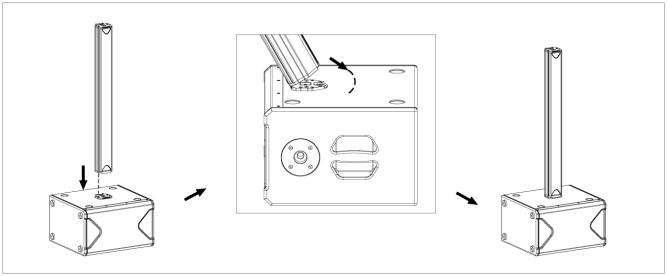
STEP 3, Position the "A" base downward, place the column speaker base in an incline and slowly position column base to match the Subwoofer connector socket. The copper positioner will affix and connect the column to the subwoofer.
