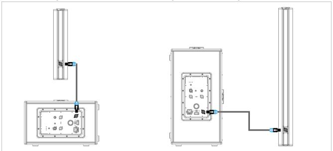
STEP 3: Use a cable with two speakon plugs to connect column speaker and subwoofer.
