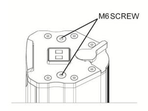
STEP 2, Take off column "A" side's two M6 screws before hoisting.
