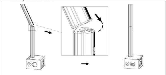
STEP 3: Ensure the additional column "A" base is down, and place the column base to match the column "B" connector socket. The copper positioner will affix to the column.
