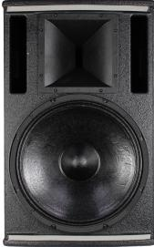
The NX15M is a compact yet high-performance two-way passive loudspeaker system. It features a 15-inch low-frequency (LF) driver with a 3-inch voice coil, and a 1-inch exit high-frequency (HF) compression driver equipped with a 1.75-inch titanium diaphragm voice coil. The NX15M's rotatable 80° x 50° HF horn ensures equal horizontal and vertical mouth dimensions, allowing precise directivity control in both planes.
