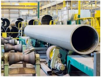
Our wheels are used in turning devices for welding and coating metal tubes, in conveyor plants for automated transport, and in cradles for internal conveyance.
