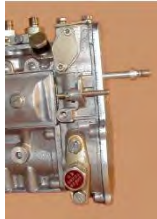
Adapter Plate From KT 175 RS-R ZEXEL Installation Kit Installed on Governor Housing
