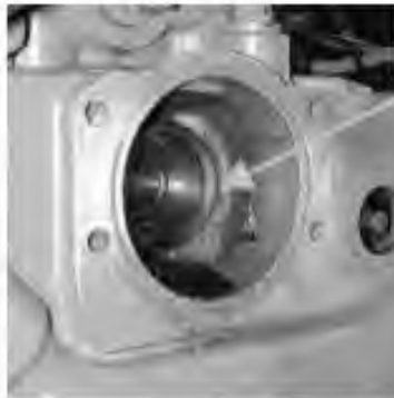
Figure 1 - Inner Bore to be Cleaned. Apply Loctite here.
