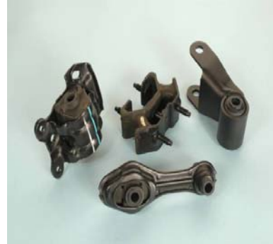
Rubber and metal suspension mountings coated with ACC ® 866
