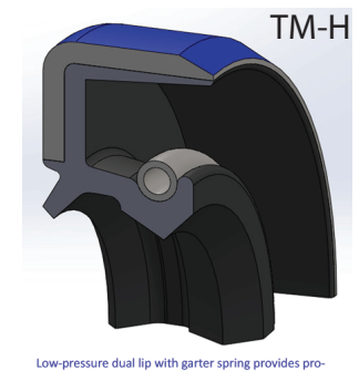
Low-pressure dual lip with garter spring provides protection from contaminants. Precision ground metal OD with a lead-in chamfer for ease of installation. Internal face of the steel case is fully rubber covered to prevent corrosion.
