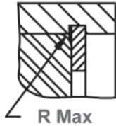
Allowable Corner Radius and Chamfer
