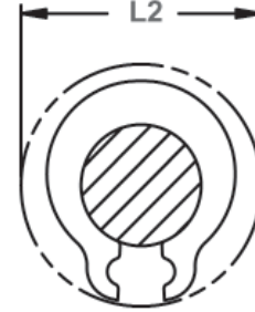
Clearance Diameter Installed on Shaft
