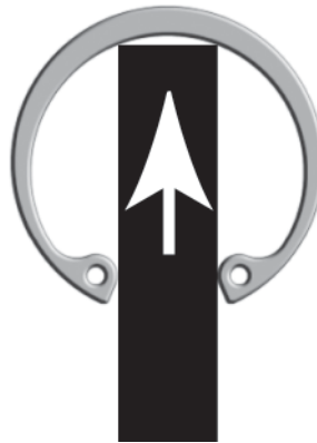
Figure A - This is the preferred way to transfer feed an internal ring into a tapered housing by inserting the mechanism between the lugs (Note: Finger thickness should be 80% of the minimum ring thickness).
