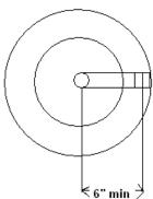
3. Rear most part of hitch must not extend behind rear plane of the tire.
