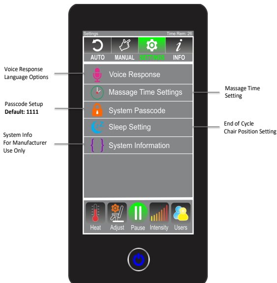
Fig.11: System Setting Description
