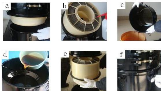
Cleaning method of oil-bath air filter
