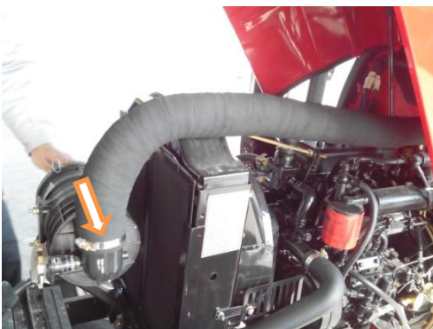
Dry-type air filter intake system clamp
