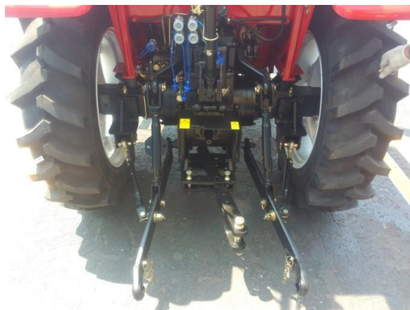
1. Swing rod 2. Connecting pin 3. Elastic lock pin of connecting pin 4. Locating pin; 5. Elastic lock pin of locating pin 6. Traction pin
