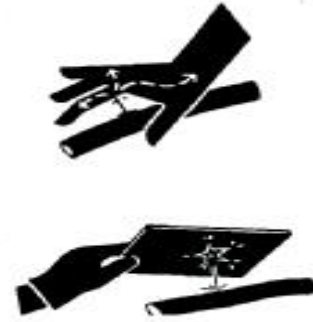
Fig. 1-9 Leakage of hydraulic pipeline
