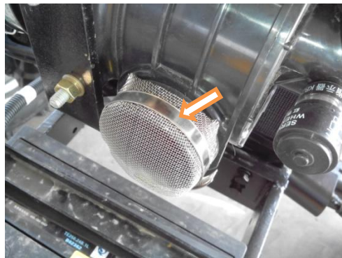
Dry-type air filter intake system clamp
