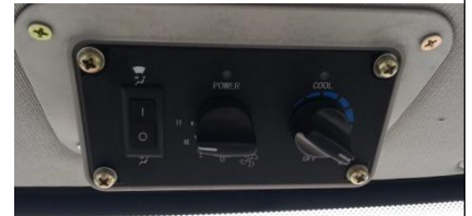
Picture 3-43Air conditioning control panel
