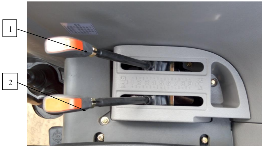
Fig.3-47 Lifting of hydraulic suspension system
