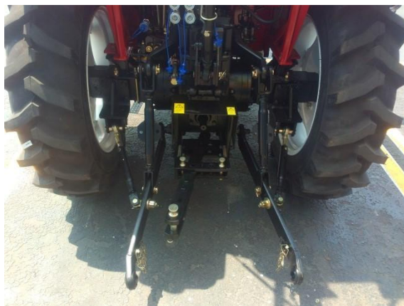
Fig. 3-61 Rightward swing of traction rod (swinging for 15°)
