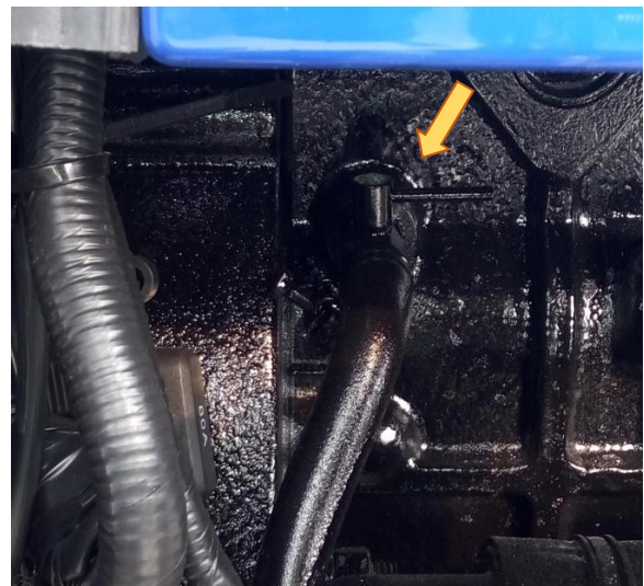
Water drain valve of cylinder
