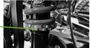
Figure 2 : Spring preload adjustment
