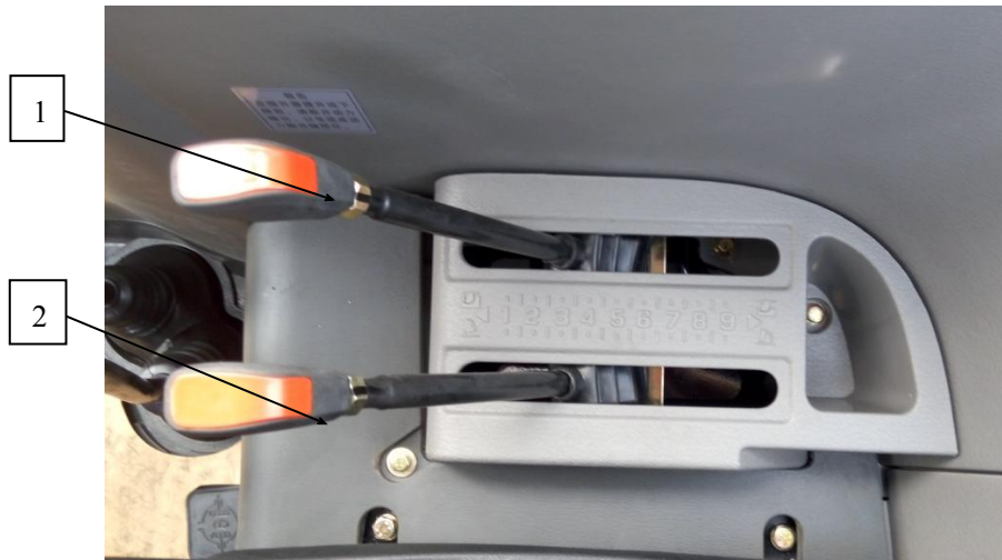
Fig.3-47 Lifting of hydraulic suspension system
