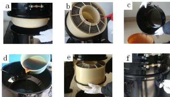
Cleaning method of oil-bath air filter
