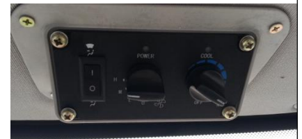
Picture 3-43Air conditioning control panel
