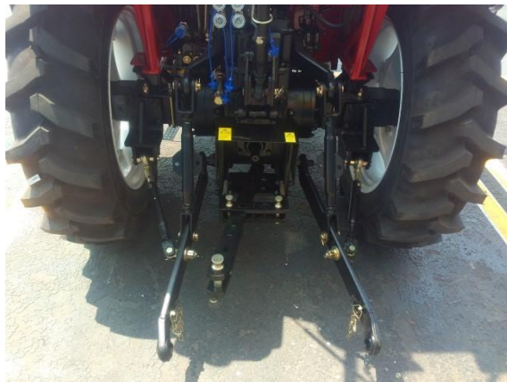
Fig. 3-61 Rightward swing of traction rod (swinging for 15°)
