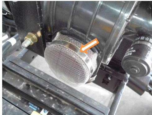
Dry-type air filter intake system clamp
