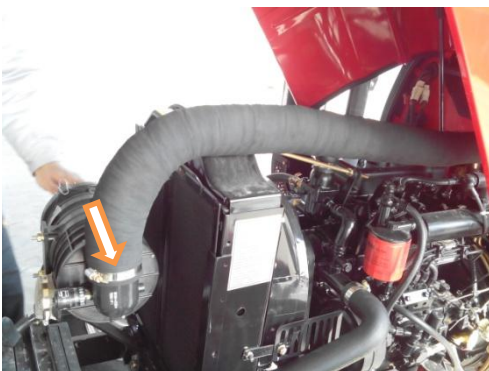
Dry-type air filter intake system clamp
