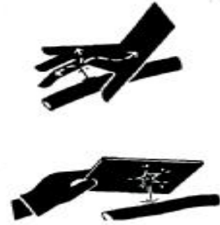
Fig. 1-9 Leakage of hydraulic pipeline
