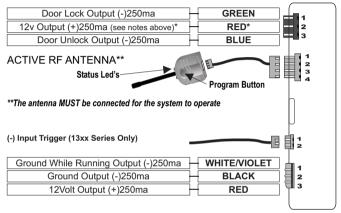
**NOTE:** The 2 pin white and 3 pin white auxiliary connectors are not available on the 32xx series.
