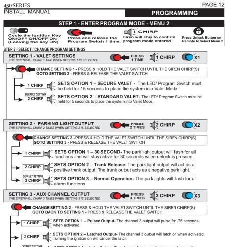
SETS OPTION 3 – Active Output- The channel 3 output will stay on as long as the button is held for a maximum of 5 seconds.
