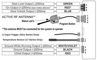
**NOTE:** The 2 pin white and 7 pin white auxiliary connectors are not available on the 42xx series.
