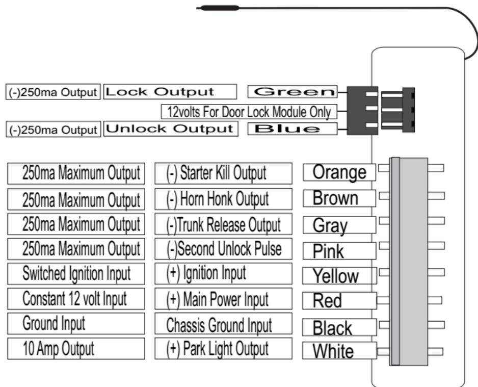
**\*The 12volt output on the keyless entry connector is not to be used for anything other than supplying power for voltage inverter's, and door lock modules such as the DL-3 and DL-7.**
