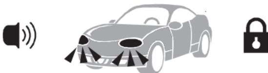
**SIREN and HAMMER ICONS-** These icons indicate that the alarm has been triggered by the shock sensor input.
