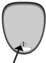
Carefully remove the screw from the back of the remote.
