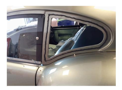
If minor adjustments are needed, slacken the M4 bolts on the side window hinges.
