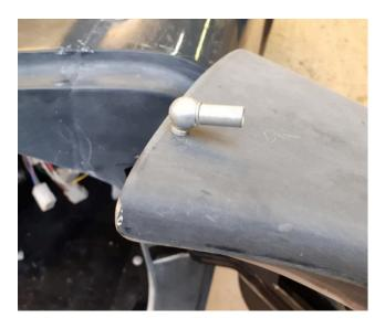
7. Install the side window and screw the depressurized gas ram into the elbow fitting on the door. Ensure you secure the hinge with the R clip to prevent the window from lifting. You can make adjustments by loosening the nuts and bolts on the hinge.
