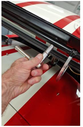
Once the window is fitted, bolt down the top of the rear window to the tailgate assembly.
