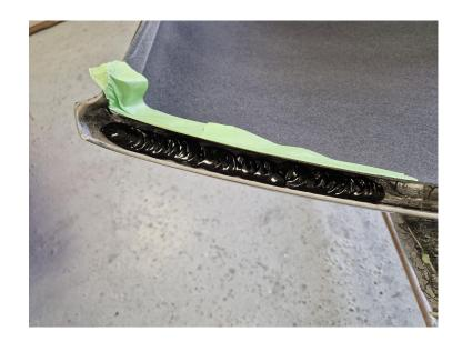
Refit the metal hardtop corners, this time using a generous amount of the adhesive provided.
