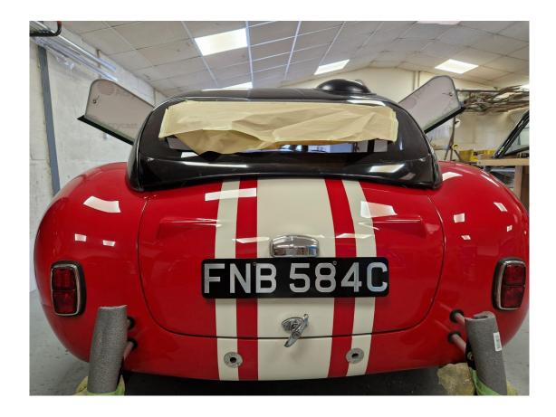
**Step 3.**Remove the Hardtop and use a step hole cutter to drill 10-millimeter diameter holes.
