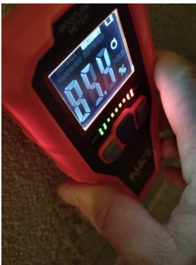
Moisture reading at the base of the foundation shows very high level of moisture.
