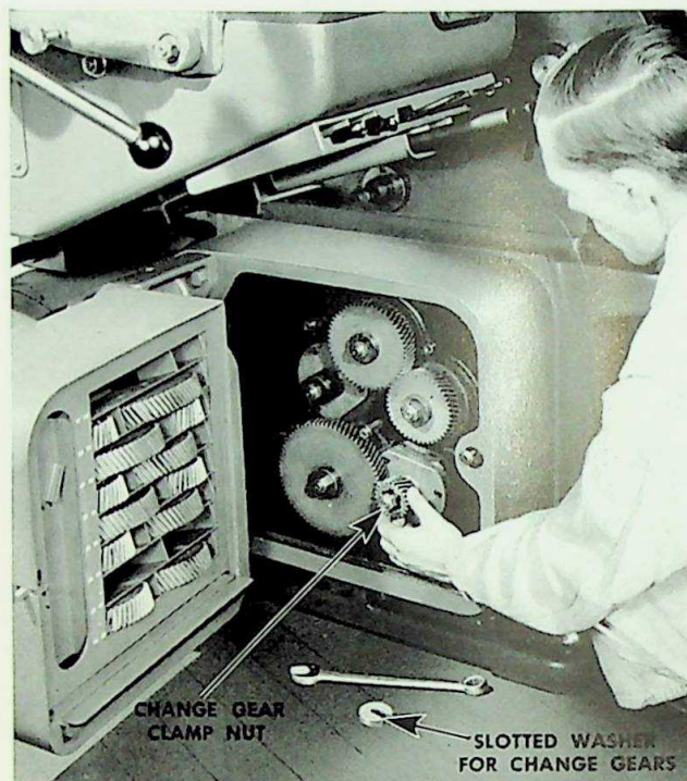
Fig. 8. Installation of Spindle Speed Change Gears.
