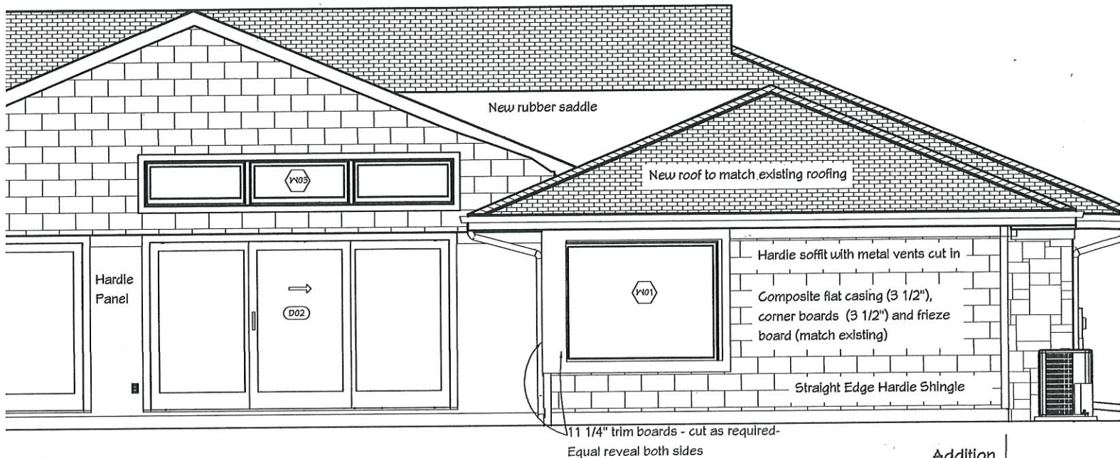
1 Proposed East Elevation 1 Scale: 1/4" = 1'0"
