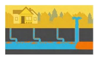
Sewer jetting also helps to eliminate and remove bacteria from sewage pipes. Due to the various materials that may travel down a drain and into a pipe, microorganisms can grow and produce an odor. Sewer jetting will remove any bacteria that has grown in the pipes through the high-pressured water and get rid of any odor that persisted because of it.
