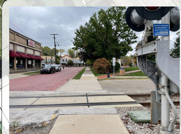
Replace 6' walk with 10' trail. Trail adjacent to curb - no impacts to park trees
