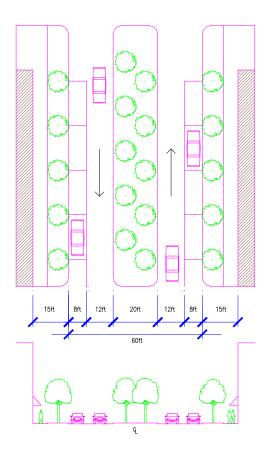
**Design Speed** 25-30 mph Min. Centerline Radius 260 ft Pavement Width (F-F) 18-14-18 ft **ROW Width** 90 ft **Curb Radius** 15 ft Drainage Curb & Gutter On Street Parking Yes (Marked) **Street Trees** Yes Sidewalks Yes
