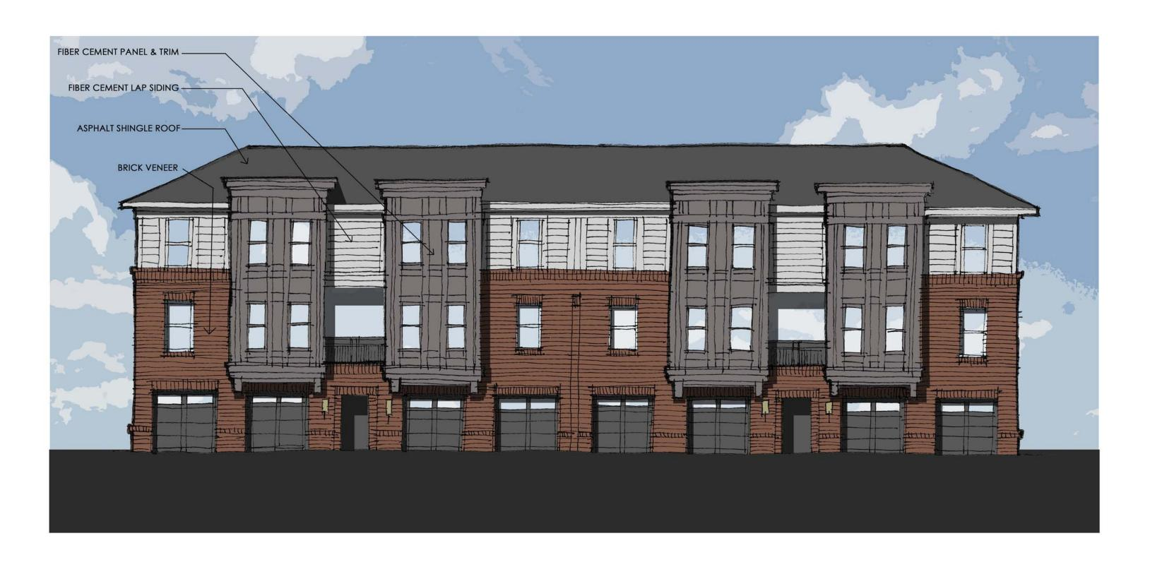
TYPICAL CARRIAGE BUILDING FRONT ELEVATION
