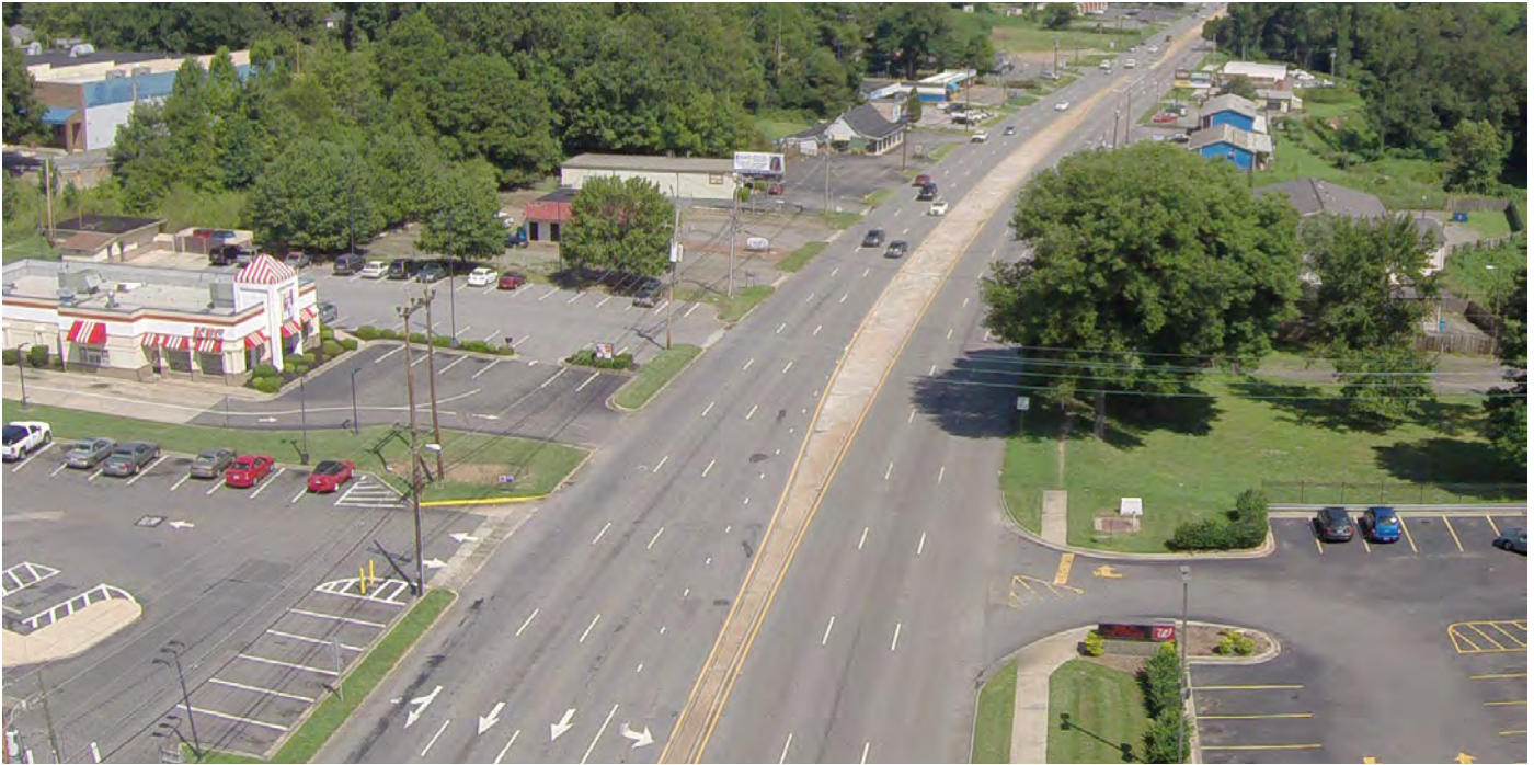
Above: Belmont’s portion of Wilkinson Boulevard hosts a range of Annual Average Daily Trips (AADT) from 16,000 to 21,000 cars a day. This is well below the capacity of a road of this size and configuration and would be considered to be underutilized from an engineering standpoint.
