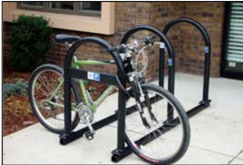
Figure 11 Inverted U racks such as the one depicted here, support the bicycle frame better and are easier to use than traditional “comb” racks, such as those that are currently being used at Belmont Central Elementary School and Belmont Middle School.
