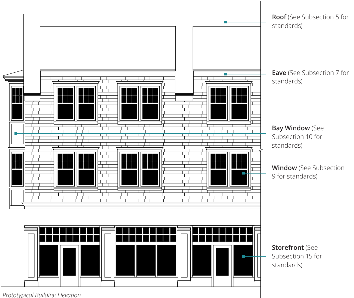
Prototypical Building Elevation
