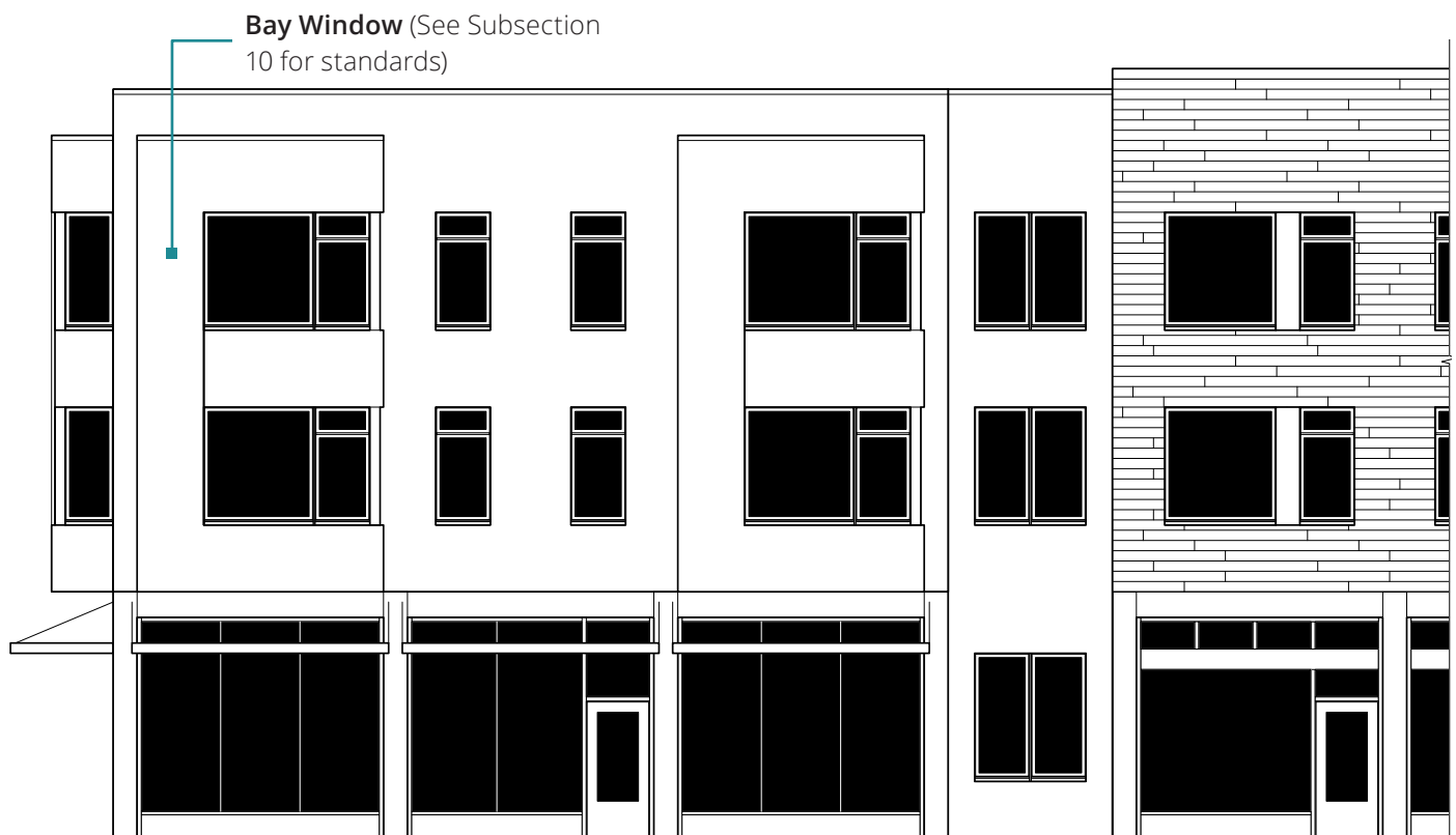
Prototypical Building Elevation
