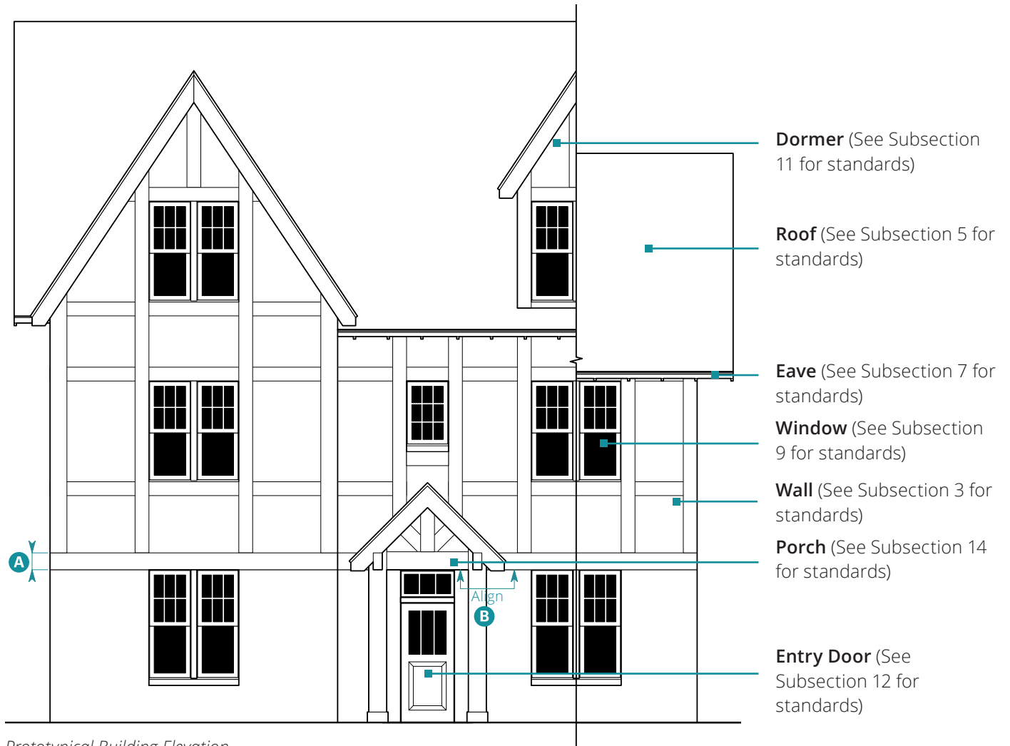
Prototypical Building Elevation
