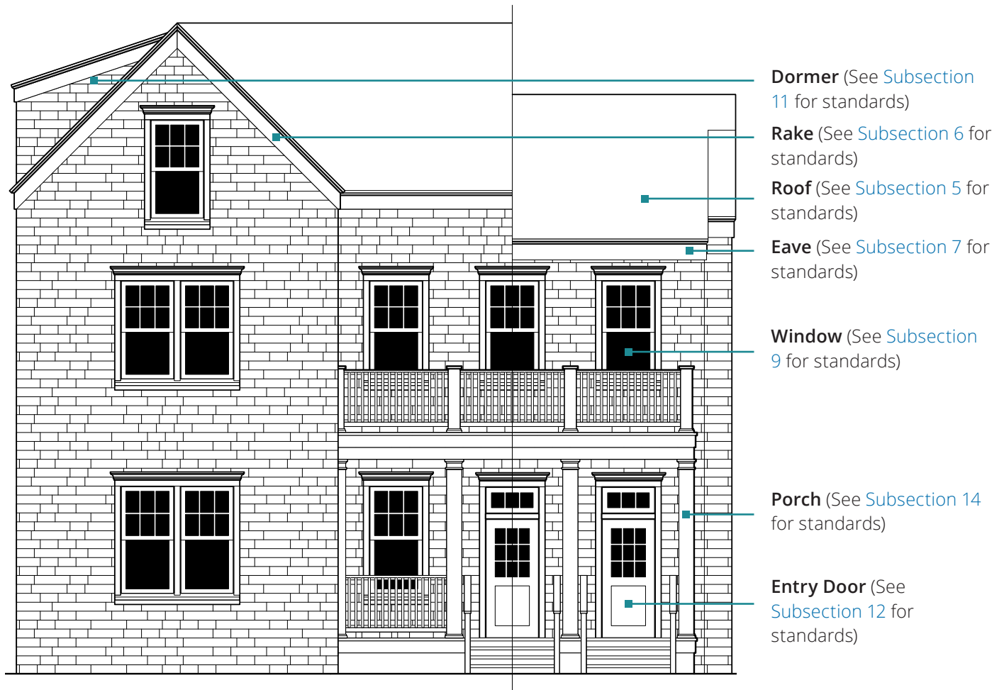
Prototypical Building Elevation
