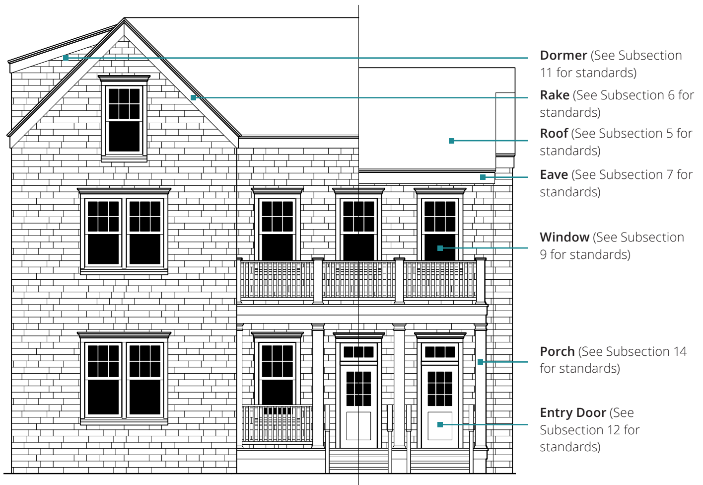
Prototypical Building Elevation
