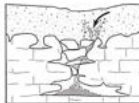
Figure 30: Cover-Subsidence Sinkhole Formation
