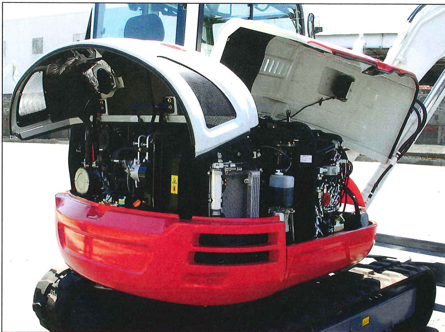
Large lockable service hoods provide vandalism protection and outstanding maintenance access.
