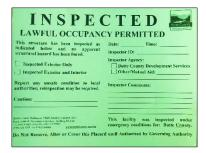
Green: The Green Placard means the structure is "Safe for Occupancy." Your structure is safe to occupy as long as it has water, electrical and gas service (if gas appliances). Structures may be damaged, yet the safety of the structure was not significantly changed by the disaster.
