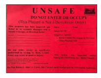
Red: The Red Placard means "No Entry." Structures are damaged and pose an imminent threat to life or safety under expected loads or other unsafe conditions. Do not enter these structures.
