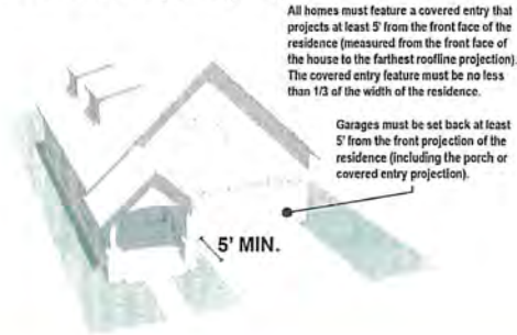
Figure 15.96.050(A) Covered entry and garage setback examples
