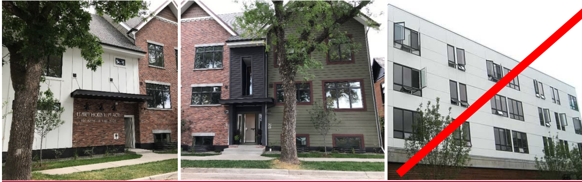
Figure 15.96.440.E Acceptable and unacceptable cement board examples.
