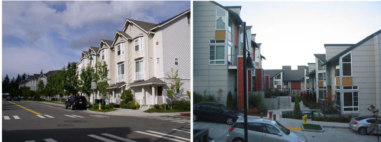
Left image – bad: Lack of color variation and setback too shallow. Right image – bad: Window style is too modern (offset corner windows).
