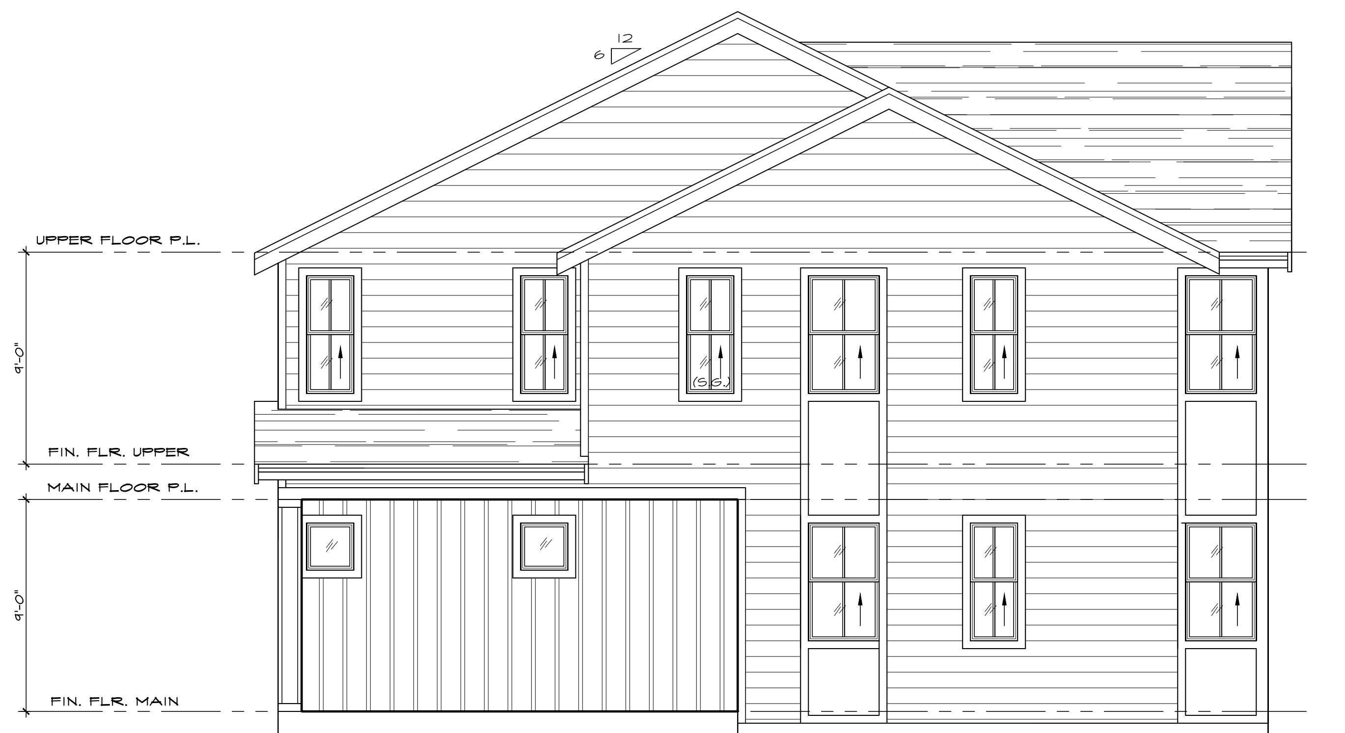
LEFT ELEVATION SEE GENERAL NOTES SCALE: 1/4" = 1'-0"
