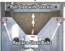
13. Attach a pulling means to the shackle on the mobile sheave assembly. (See Fig. 6)
