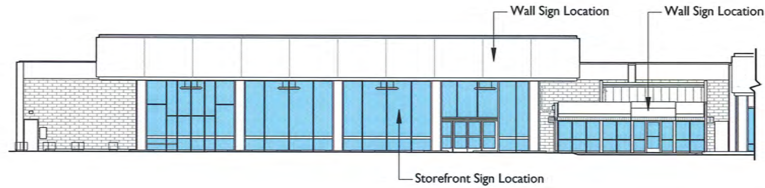
BUILDING C - WEST ELEVATION
