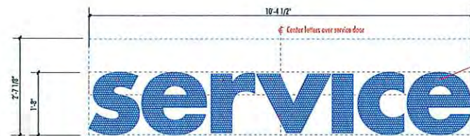
CM-S-CL26 INDIVIDUAL LED ILLUMINATED CHANNEL LETTERS (ONE SET REQ'D) Scale: 3/4" = 1'-0" 28.91 SF
