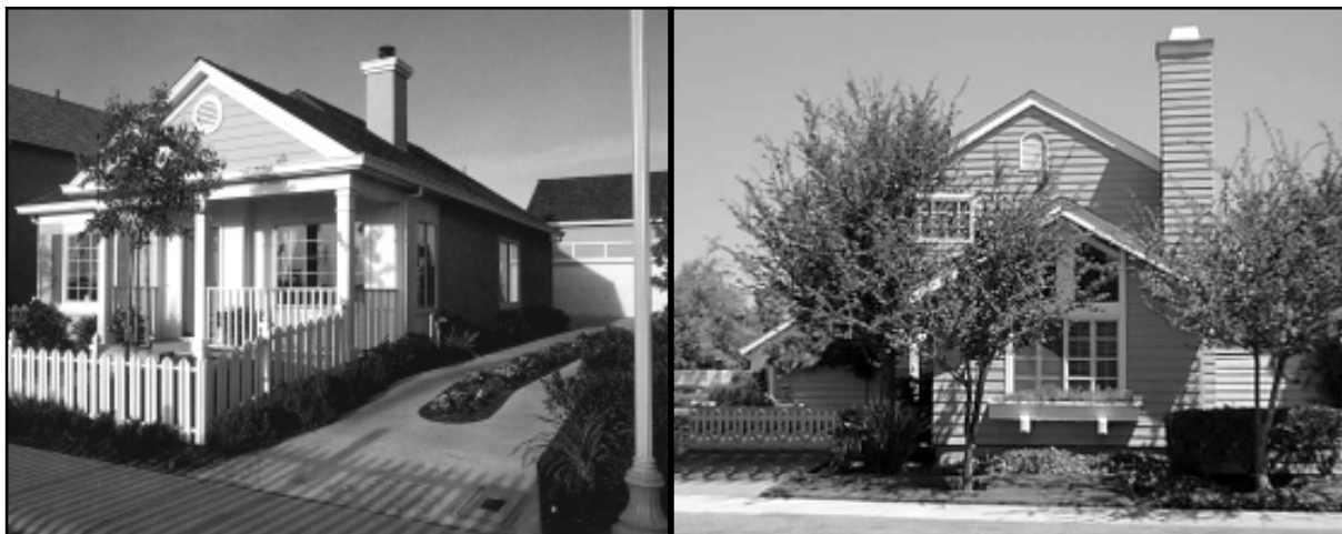
Examples of new housing suitable for Sterling Park infill. Requirements for this area include pitched rooflines, one and two-story average height, and building surfaces well articulated with windows, doors, balconies, bays, exposed beams, and overhangs. These examples also have recessed garages, which help improve the appearance of the street.
