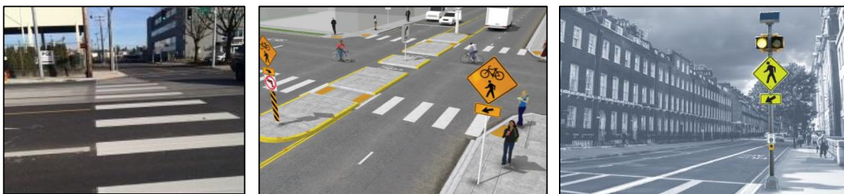
Figure 17: Example of Enhanced Pedestrian Crossing
