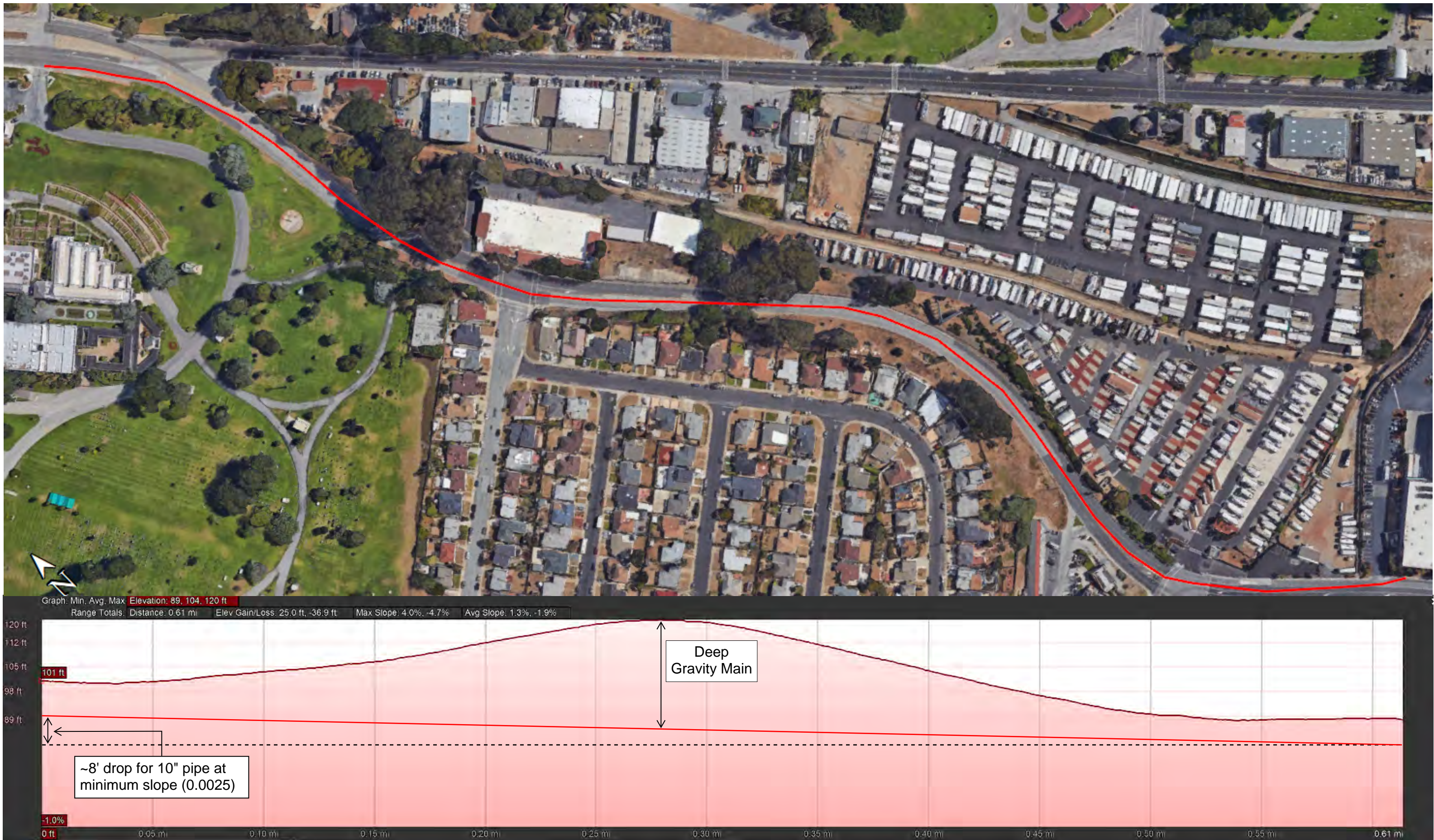
Figure 9-4. Alternative 2: Gravity Main on El Camino Real Plan and Profile Views
