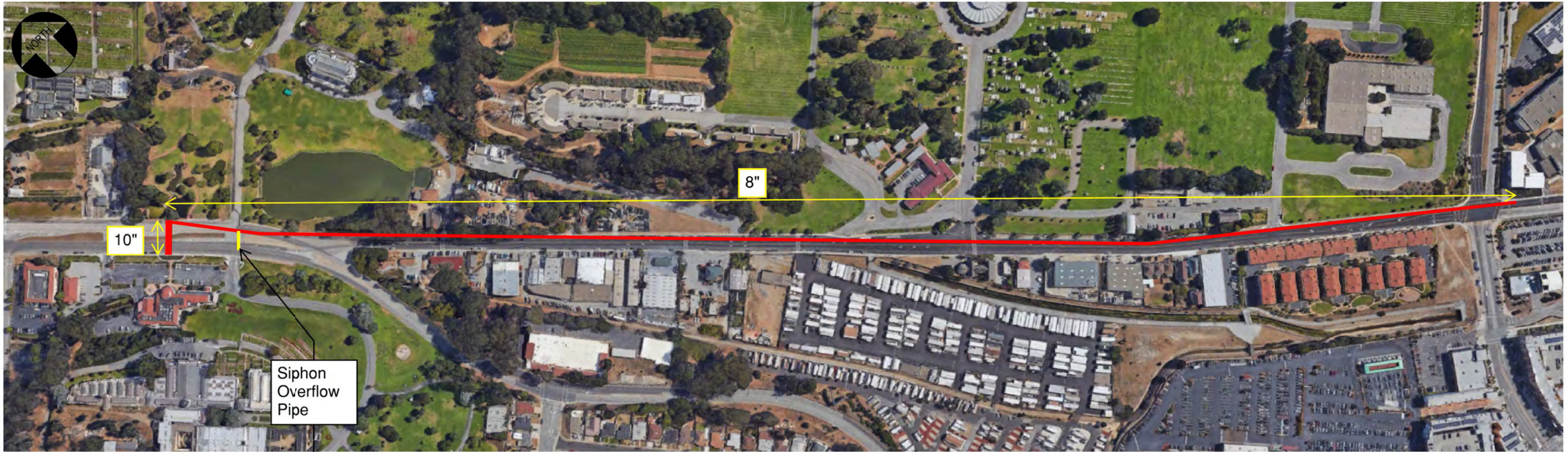
Figure 9-3. Alternative 1: Parallel Gravity Main on Mission Road Plan and Profile Views
