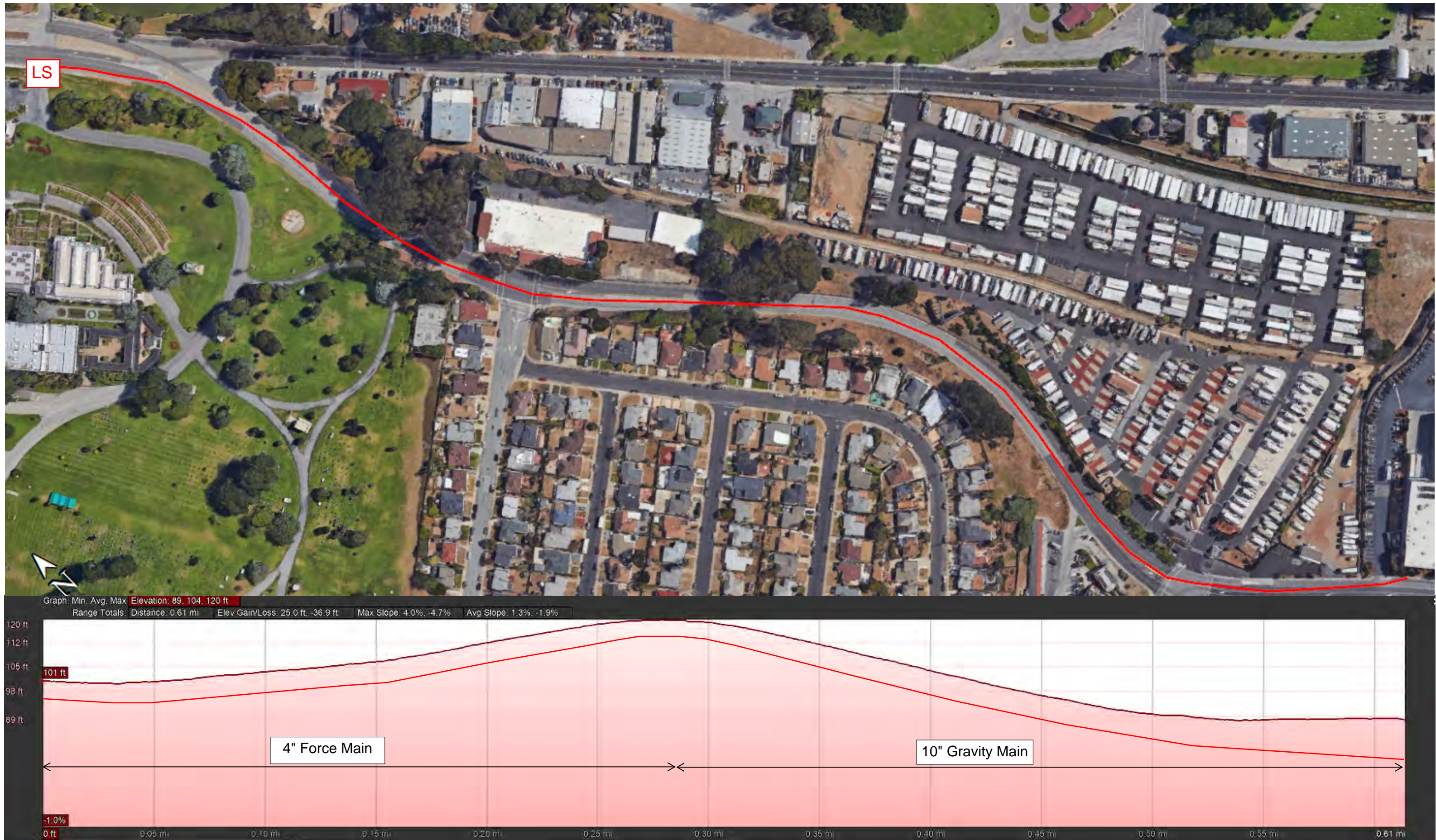
Figure 9-6. Alternative 3B: Lift Station and Force Main on El Camino Real Plan and Profile Views
