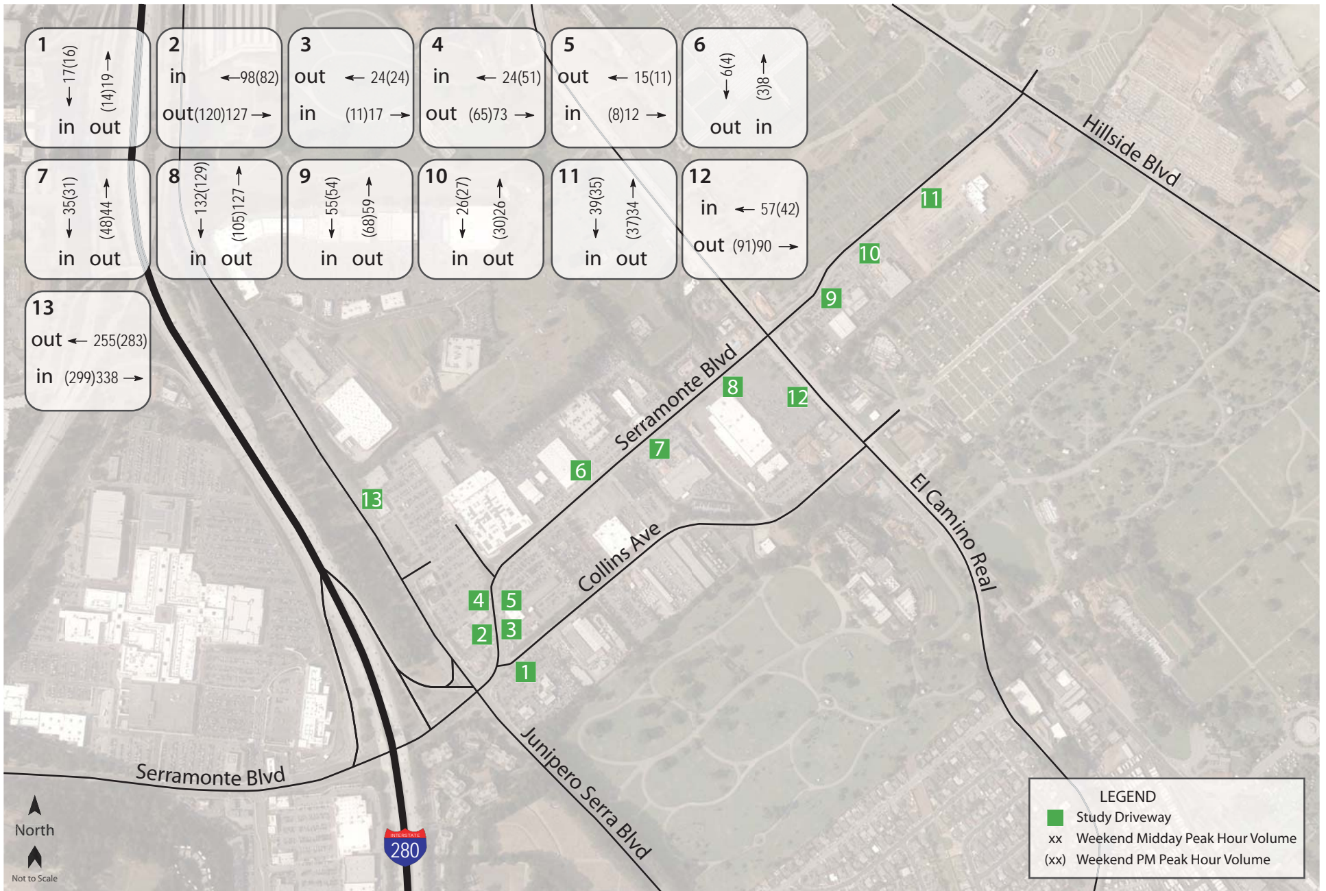
Serramonte Boulevard/Collins Avenue Master Plan Figure 6 – Existing Weekend Driveway Ins and Outs
