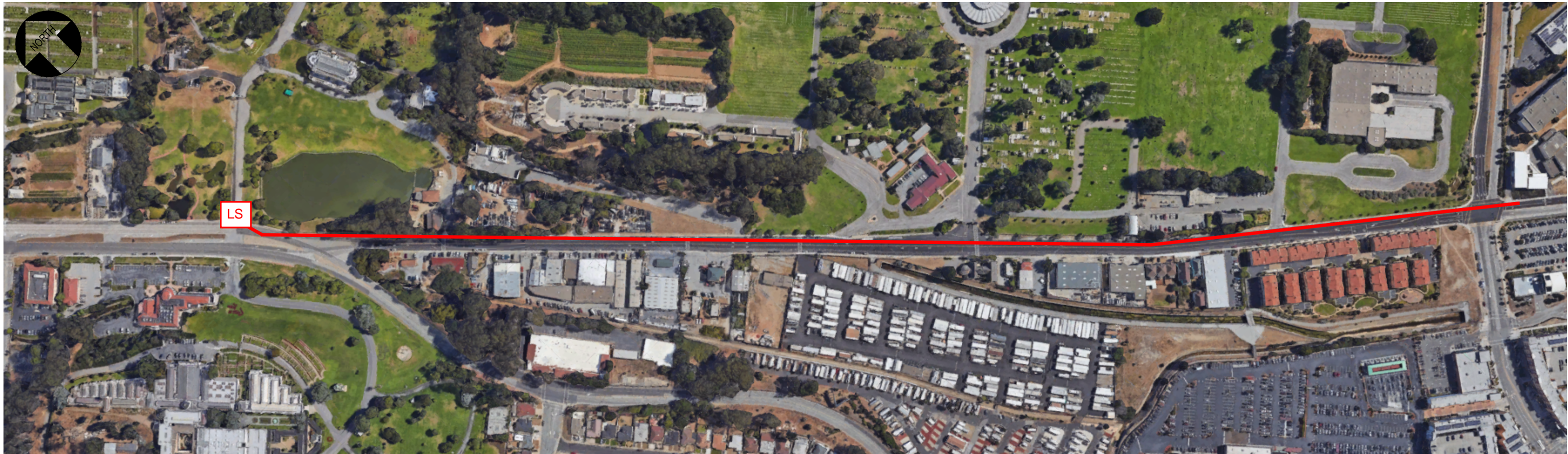
Figure 9-5. Alternative 3A: Lift Station and Force Main on Mission Road Plan and Profile Views
