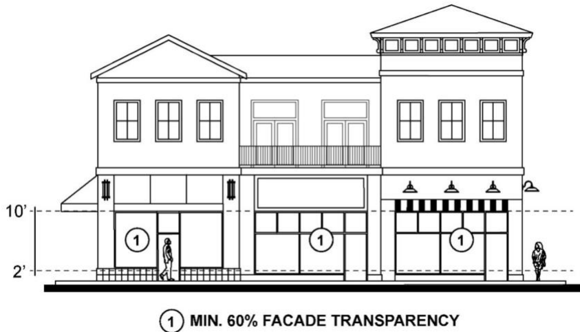
FIGURE 8: MIXED USE FAÇADE TRANSPARENCY
