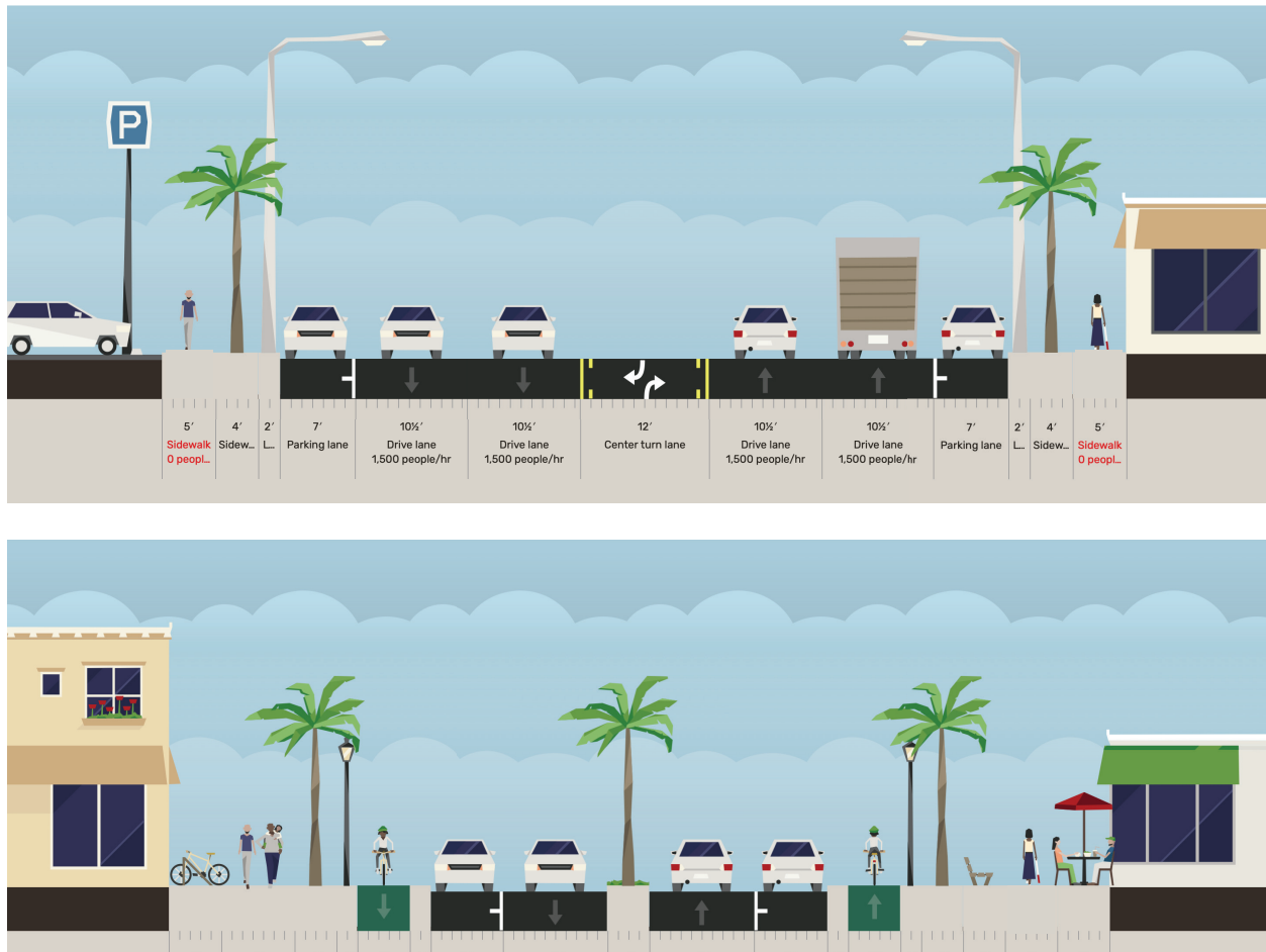
Figure 1: A car-oriented design (top) prioritizes the throughput of vehicles, whereas a person-oriented design (bottom) prioritizes the comfort and safety of all users.
